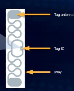
**Tag IC** The heart of the tag – the RFID silicon chip
